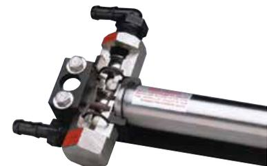
E-Z Meter Pumps with the double ball, built-in check valves provide better performance by virtually eliminating air locking. Available in 316 stainless steel or Teflon™ cylinders.
