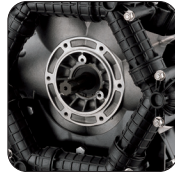
C/C Version 1 3/8" 6 Splined Thru Shaft
