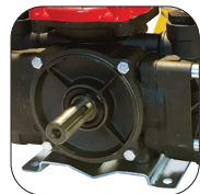
SP/SGC Version Straight 3/4" Keyed Shaft 1/2" BSP threaded outlet flange
