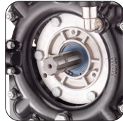
C/C Version 1 3/8" 6 Splined Thru Shaft
