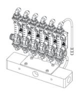
VisaGage II Kits when just adding flow monitors to your 1770NT John Deere® Planter (planters built 2012 and after). Kits will bolt directly to your manifold.
