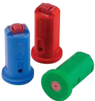
The Albu<sup>z</sup>® AVI Twin (ATW) brings drift control and coverage together. Using proven AVI technology, the AVI Twin draws air into the nozzle, mixing it with the spray to create a twin spray of drift resistant air-filled droplets. Drift is greatly reduced, spraying the canopy with dual trajectories to improve coverage.
