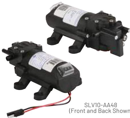
The Shurflo SLV is ideal for low volume, intermittent-duty applications requiring a compact pump with low power consumption. Unique design has no metals in the fluid path for maximum chemical resistance. Pump features include automatic demand operation and elastomers that handle a wide variety of chemicals. Perfect for low volume spraying and transfer. Cost effective yet with high performance and reliability; the SLV offers tremendous value.
