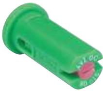
The Albu<sup>z</sup>® AVI-OC air-inducing Venturi off-center ceramic spray nozzle with air suction provides large, air-filled droplets that burst on impact with target.
