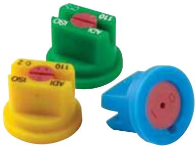
The Albus® ADI anti-drift spray nozzle provides a versatile balance of drift reduction and target coverage. The proven pre-orifice design creates droplets that are well suited for a wide range of spray applications. The ceramic orifice resists wear better than other materials and will provide acre after acre of service.
