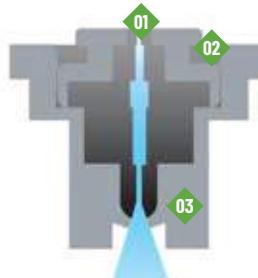
01. Non-Air Inducted; Pre-orifice design for excellent performance with suspension solutions
