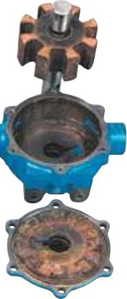
These three pump housings were photographed after being tested with a 30:1 mix of water and Roundup® herbicide.
