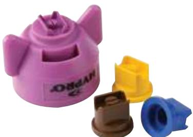
Variable Pressure nozzle maintain a consistent spray angle over a wide pressure range down to 20 PSI (1 BAR) and are available in 80° and 110° versions to work with different boom heights.
