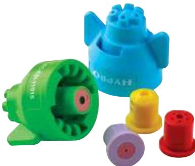
The ESI six stream nozzle is designed for applying liquid fertilizer. It creates six individual streams that distribute the fertilizer on the soil while getting less on the crop. The wear resistant metering orifice and unique low pressure distribution chamber keep the streams stable to reduce atomization and prevent leaf burn and scorching. Spacing and spray height is similar to 110° broadcast nozzles.
