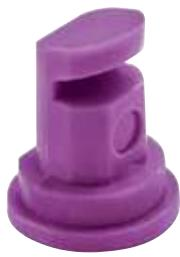
The DeflecTip and PoliJet wide-angle flood fan nozzle creates a wide pattern at very low pressures while creating mainly medium and coarse droplets. It is well suited for sprayers using very low pressures, including manual sprayers.
