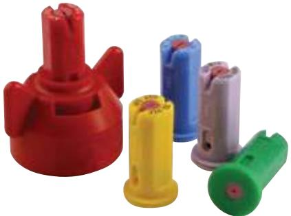
The Albuze® AVI draws air into the nozzle and mixes it with the spray to create very coarse droplets that minimize spray drift. The air-filled droplets have a larger footprint on the leaf than similar non-air droplets and hold to the leaf for better control. Durable Albuze ceramic orifice create the longest wearing spray nozzle of its kind.
