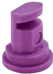
The DeflecTip wide-angle flood nozzle creates a wide pattern at very low pressures while creating mainly medium and coarse droplets. It is well suited for mounting on machinery where a wide angle or a low spray height is desired and on sprayers using very low pressures, including manual sprayers.
