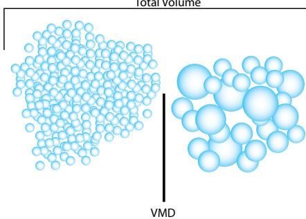
VMD is the droplet size at which 50% of the spray volume is in droplets larger than the VMD and 50% of the volume is in droplets smaller than the VMD (adapted from Matthews 1992).
