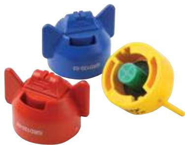
Guardian spray nozzles are ideal for insecticide and fungicide applications especially when used with suspension based adjuvants. The Guardian's unique 20° inclined spray pattern allows users to aim the spray rearward for general spraying, forward for vertical targets, or alternate nozzles to create a twin spray.
