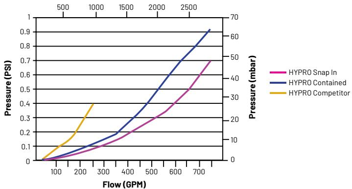
As depicted in the graph above, the Hypro Labyrinth Breather consistently performs at a higher fill rate and lower pressure than the typical competitor.
