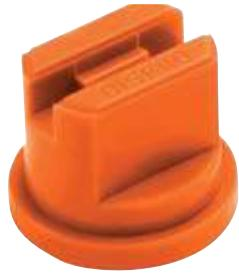
The FanTip is a general spray nozzle that produces a mixed droplet spectrum over the 30-60 psi (2-4 bar) operational pressure range. It is good for broadcast applications.
