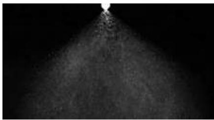
80° or 110° wide spray patterns; broad flow range and droplet spectrum to fit many spraying applications.
