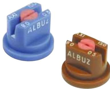
The AXI 80° extended range fan pattern nozzle can be used for directed applications of a variety of chemistries and products. They are well suited to applications where smaller droplets are favored. They are equipped with a ceramic orifice to provide long-lasting performance.
