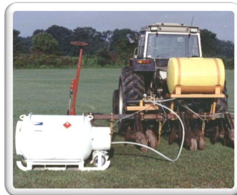
RF809-4 Little Squirt Self Contained 12Volt Fumigation Pump System
