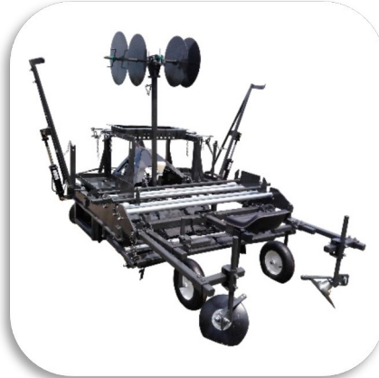
RMC-172 Mulch Layer w/Hyd Machine for Raised Bed Mulch Applications up to 66" Width
