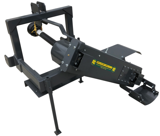
Off-Set Ditcher with Chain Drive & Clutch • 655 lbs. D6-OS-C $ 4425.00
